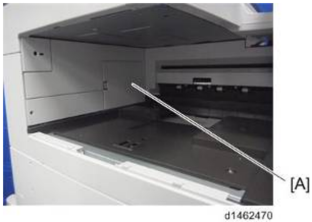
12. Paper output lower cover [A] (🔩 x3).
